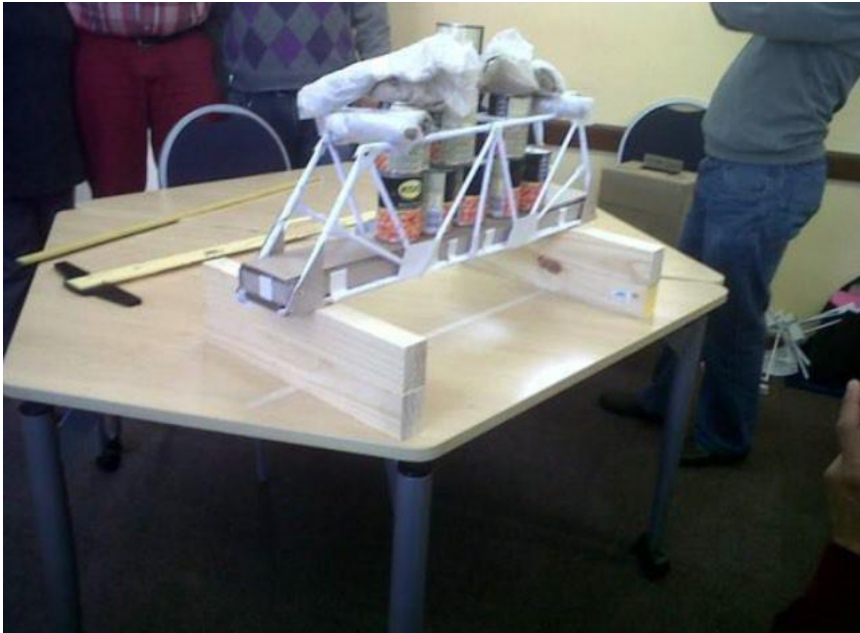
Figure 4.2: This photograph was included in a Technology teacher's portfolio as evidence of learners engaging in the technology design process during a post-intervention class in which the teacher applied the knowledge and skills gained through the short learning programme. Here the learners tested the strength of their constructed bridge.
