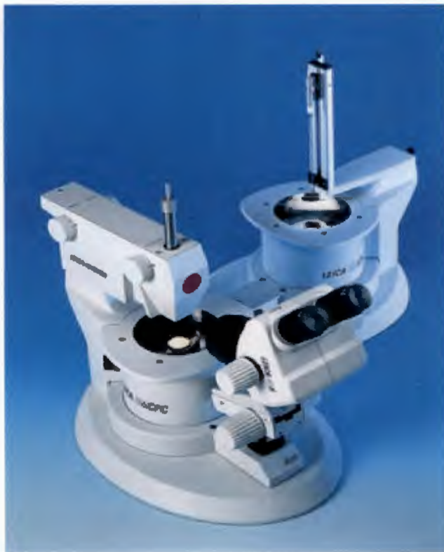
Figure 2.4. The Leica EM CFC-Cryo-workstation that is used for Plunge Freezing (Immersion Cryofixation)
