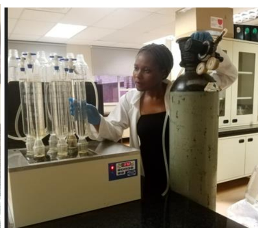
Six Composition tanks filled with slurry (400ml)
