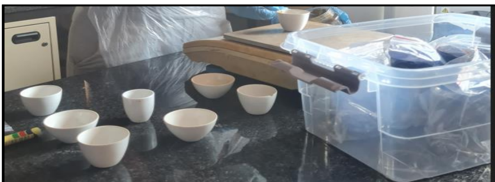
Figure 5.2: Preparing and weighing the substrate and crucibles
