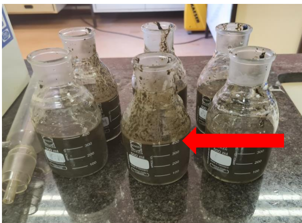
Six Composition tanks filled with slurry (400ml)
