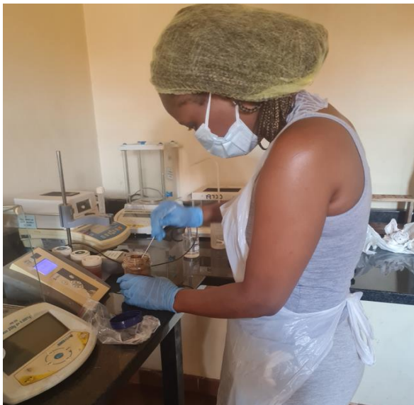
PH testing of Substrate
