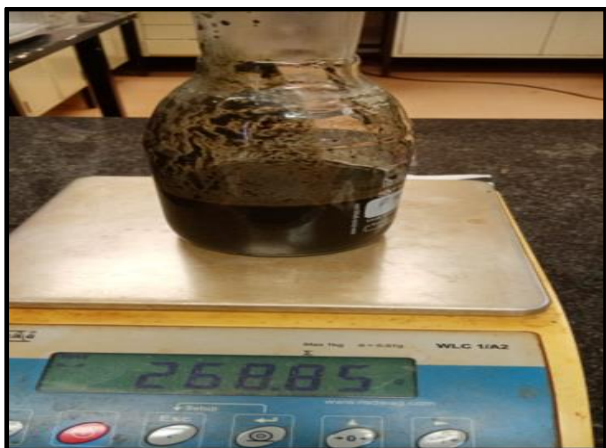
Figure 5.5: The inoculum (268,85 g) for the anaerobic digestion process
