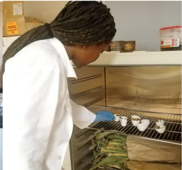
Substrate placed in the oven, 24h period
