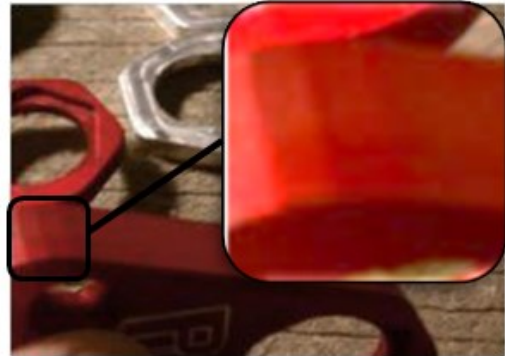
Figure 2-21: Faceted surfaces due to the software influences (CNC cookbook, n.d.)
