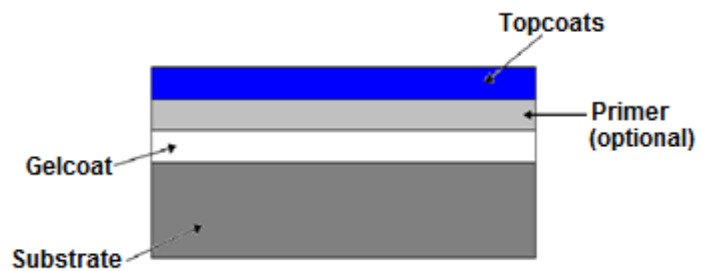
Figure 2-7: Composite surface layers (TIA, 2012).
