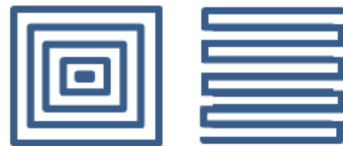
Figure 2-16: (Left) Contour offset. (Right) raster offset (CNC cookbook, n.d.)
