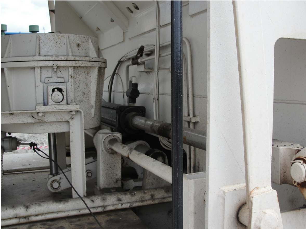
Figure 67 – Pneumatic cylinder used to operate train doors at Mine D
