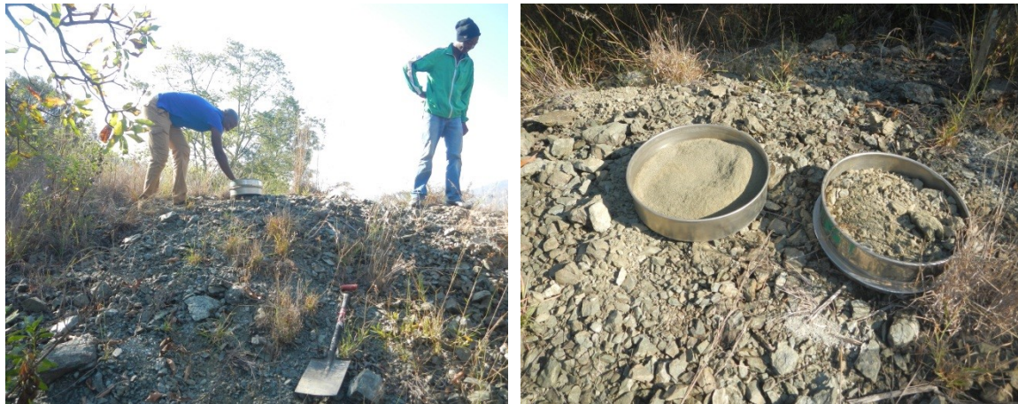
a) Sieving waste rock sample using Labotec 200mm test sieve of 2.0 mm mesh size
