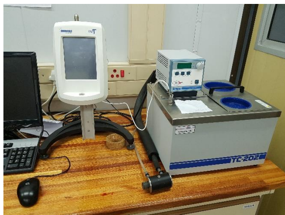
Figure B.12: A Brookfield Viscometer DV2T LV Ultra connected to a water bath
