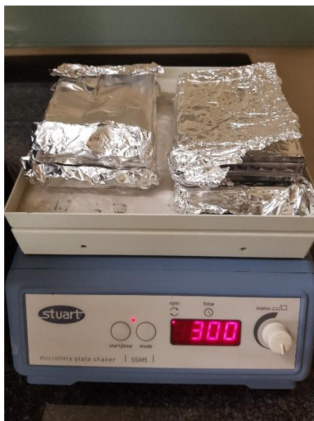
Figure E.4: Plate shaker adjusted to 300 rpm
