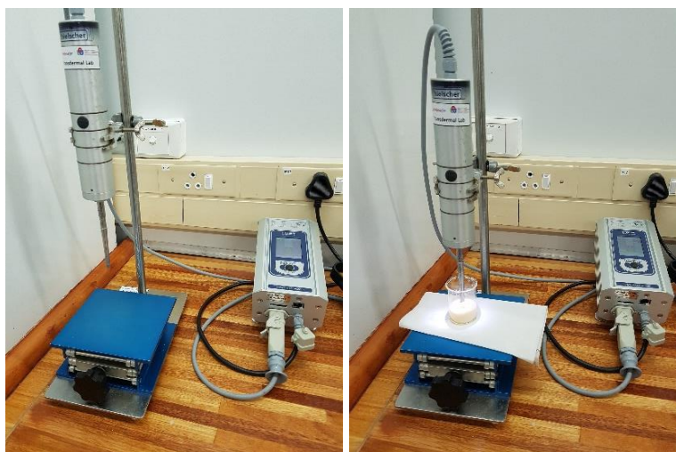
Figure B.1: High-energy emulsification method ultrasonicator (Model UP200St)
