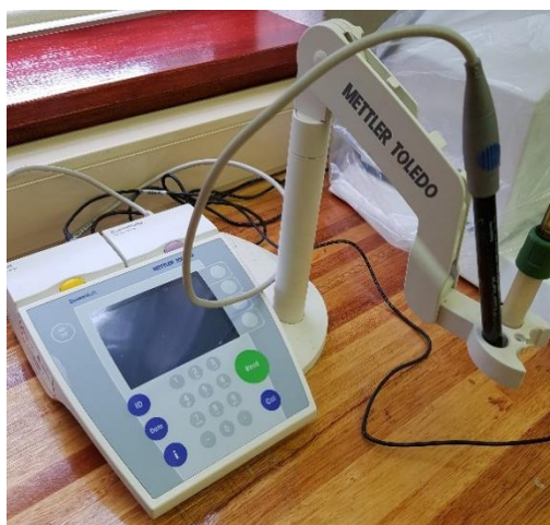
Figure B.4: A Mettler Toledo® pH meter with a Mettler Toledo® InLab® 410 electrode
