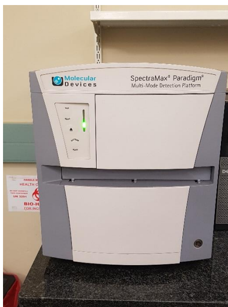
Figure E.3: SpectraMax® Paradigm® Multimode Microplate reader (Molecular Devices, United States) used to measure absorbance
