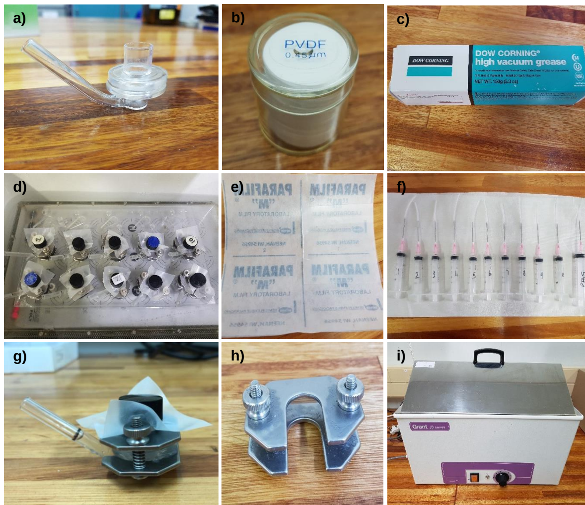
Figure D.3: Materials used for membrane release studies: a) Franz cell with a donor and receptor compartment; b) PVDF synthetic membranes; c) Dow Corning® high vacuum grease; d) Franz cells in a Franz cell stand on the magnetic stirring plate; placed in the water bath; e) Parafilm® used to cover the Franz cells; f) syringes used for extraction of receptor phase; g) assembled Franz cell with 1 ml formulation in the donor compartment (top) and 2 ml PBS (pH 7.4):10% ethanol in the receptor compartment (bottom) before placed in the water bath; h) horse shoe clamp used to fasten the Franz cell compartments; i) Grant® water bath
