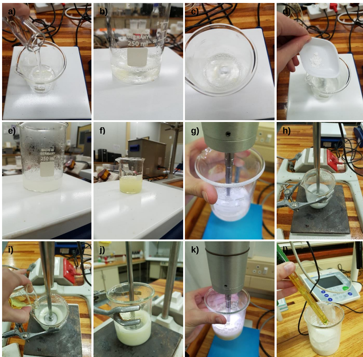
Figure C.1: Method of formulating a nano-emulgel: a) water phase preparation by adding Milli-Q® water with Tween® 80; b) mixing of Milli-Q® water and Tween® 80; c) dissolving Tween® 80 in Milli-Q® water; d) addition of the gelling agent (Carbopol® Ultrez 20) to the water phase; e) high speed mixing of gelling agent into the water phase for dissolution; f) dissolving Span® 60 into the grapeseed oil, after which API is added and dissolved; g) ultrasonication of the water phase with gelling agent (3 min); h) water phase is then placed in the overhead mechanical stirrer; i) oil phase is added to the water phase while stirring with the overhead mechanical stirrer; j) oil and water phase is left on the mechanical stirrer for 15 min; k) after 15 min on the overhead mechanical stirrer, the emulgel formulation is ultrasonicated for 5 min; l) adjustment of the pH to that of the nano-emulsion to obtain a emulgel formulation
