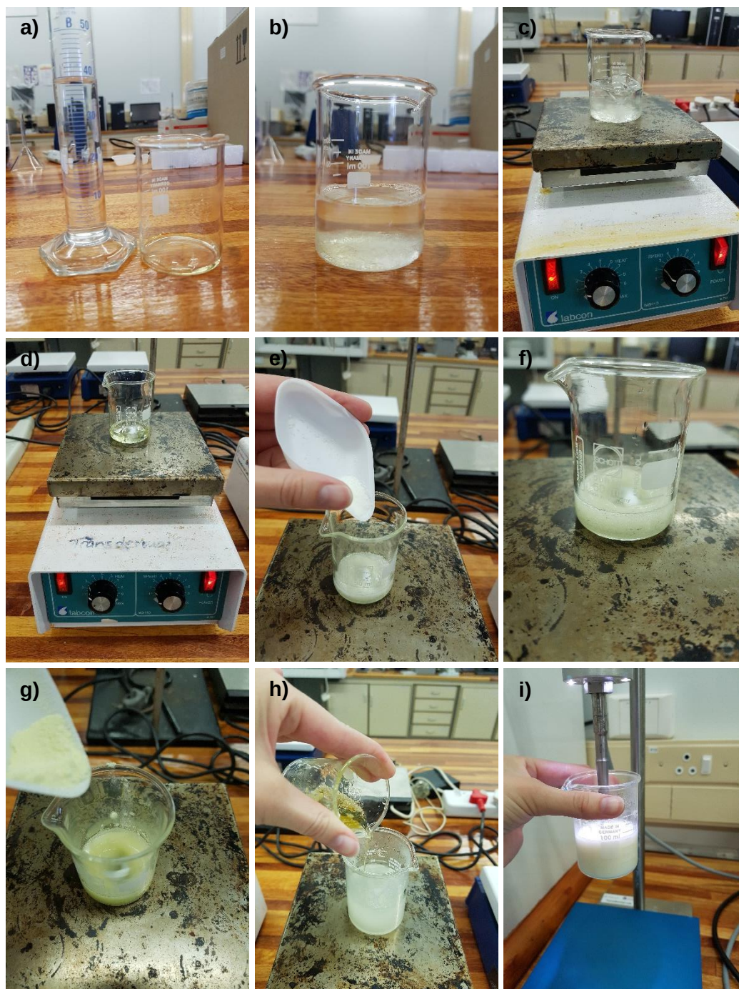
Figure B.2: Formulation method of the (NE1) : a) Tween® 20 and water measured separately; b) Tween® 20 and water mixed together; c) Tween® 20 and water pre-heated (phase B); d) grapeseed oil preheated; e) Span® 60 was added to the preheated grapeseed oil (phase A); f) heated and dissolved grapeseed oil and Span® 60; g) API is added to phase A and dissolved; h) phases A and B were mixed together; i) sonication of emulsion for 3 min in 1 min intervals
