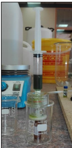
Figure 5.10: The process of sampling of extractions. The extraction is added into the syringe part of the syringe-prefilter-filter system, through which the sample is then filtrated into a HPLC vial by pushing down on the shaft of the syringe.
