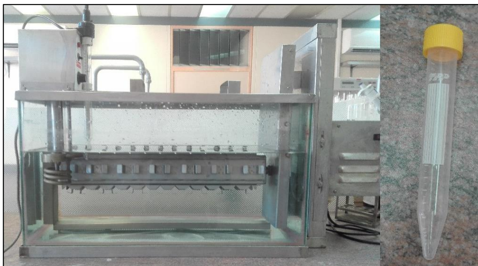
Figure 5.7: The water bath used for extractions (a) and a test tube which is to be inserted into one of the water baths circulator slots (b).
