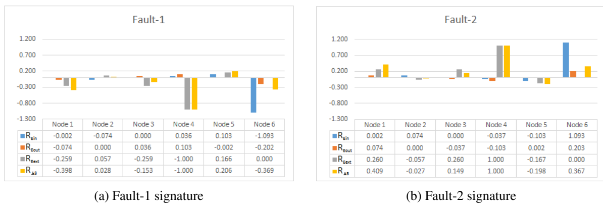
Figure 6.1: Residual-based signatures for Fault-1 and Fault-2
