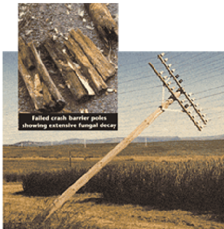
Fig 4.3; Wooden pole breakdown due to lack of preservation
