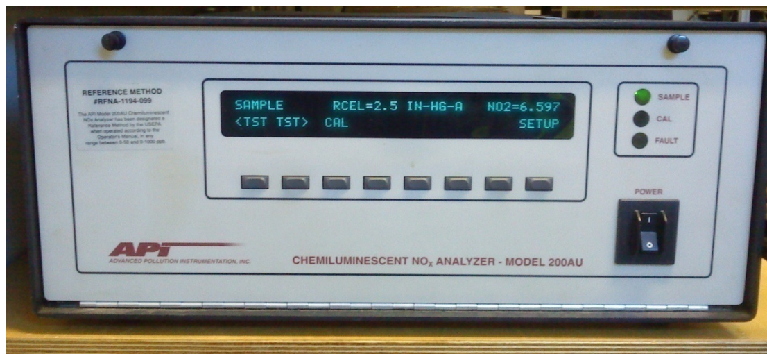
Figure 3.4: The chemiluminescent NO/NO x analyser
