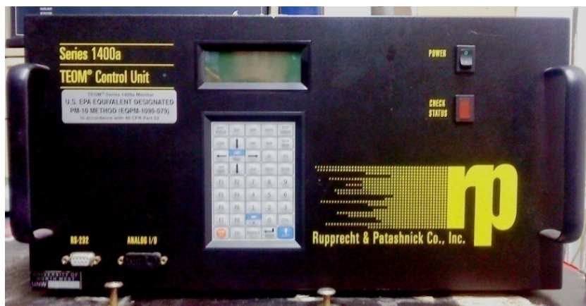
Figure 3.9: The TEOM 1400ab used to measure PM_{10} in the period 20.7.2006-11.2.2009
