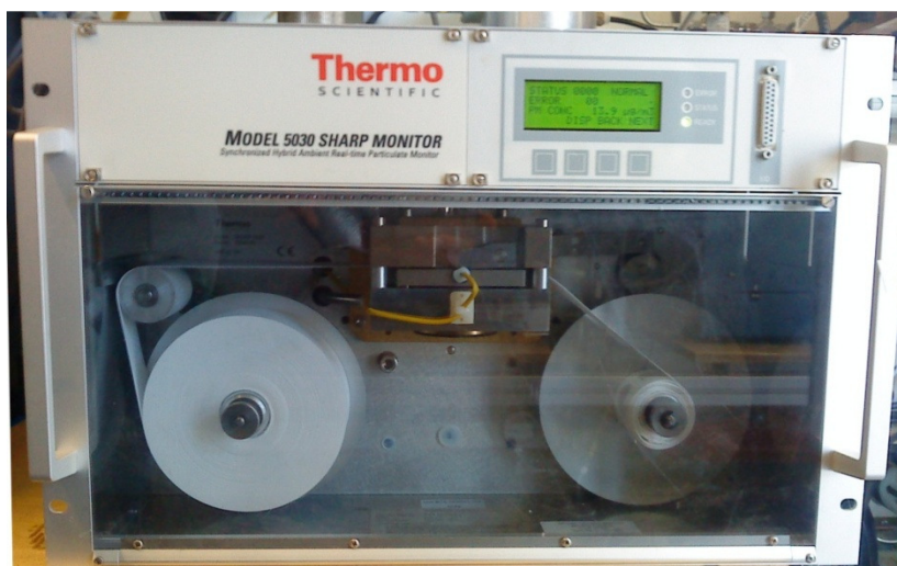
Figure 3.10: The SHARP 5030 used to measure PM_{10} in the period 12.9.2009-17.5.2010
