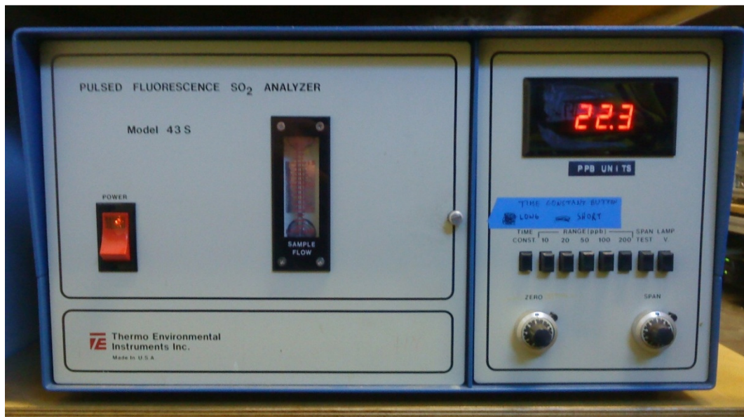
Figure 3.2: The pulsed fluorescence SO 2 analyser
