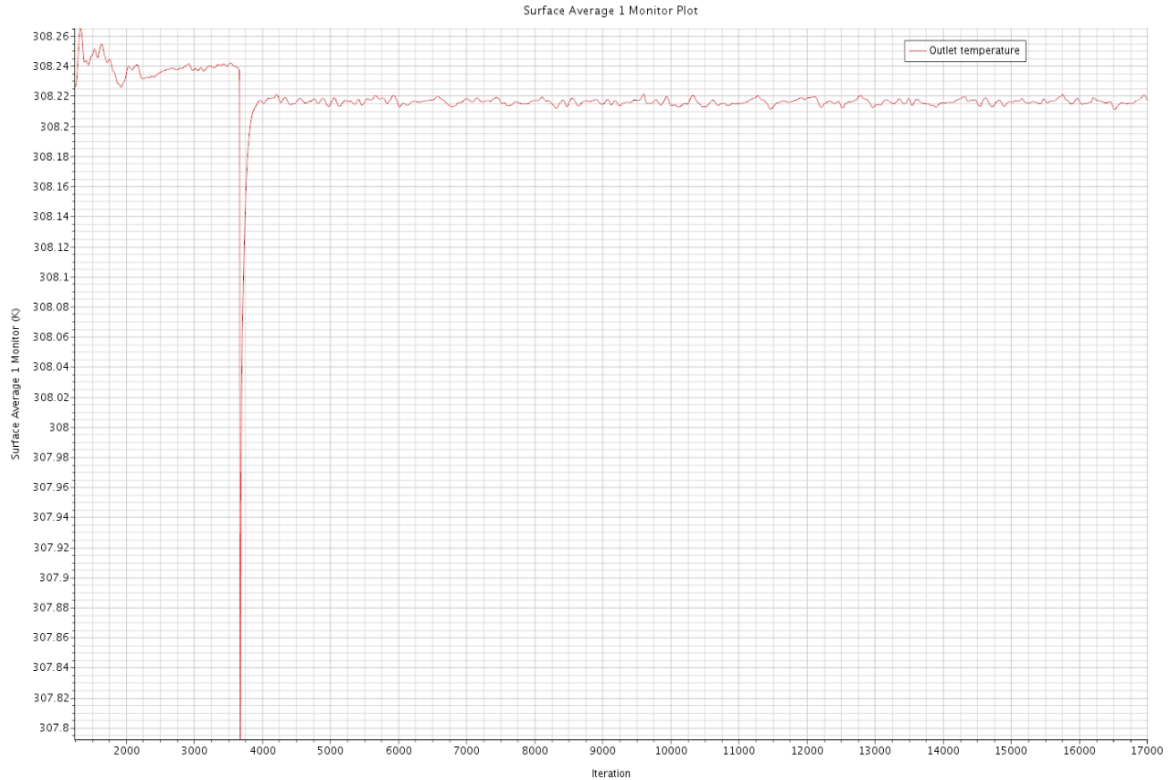
Figure C-13. Outlet temperature monitor for Mesh 2.
