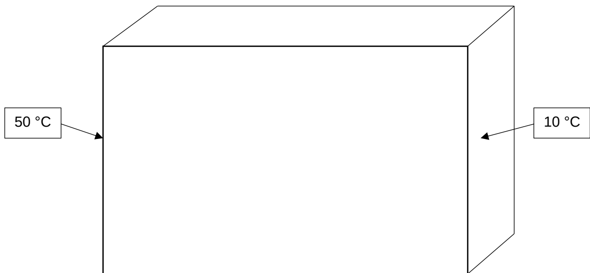
Figure 5.1-3. Air-filled cavity geomtery.
