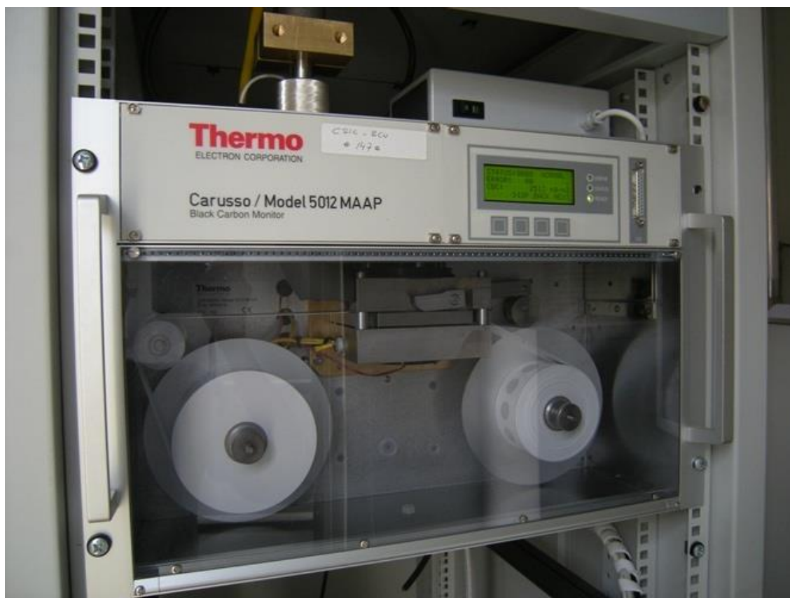
Figure 3.8: An image of the MAAP instrument used to measure eBC at 637nm wavelength in this study
