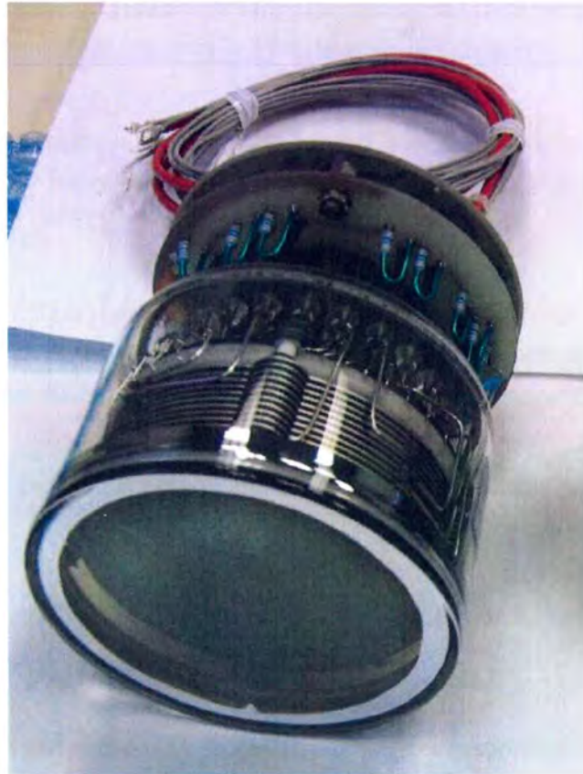
Figure 3.7: The Position Sensitive Photomultiplier Tube
