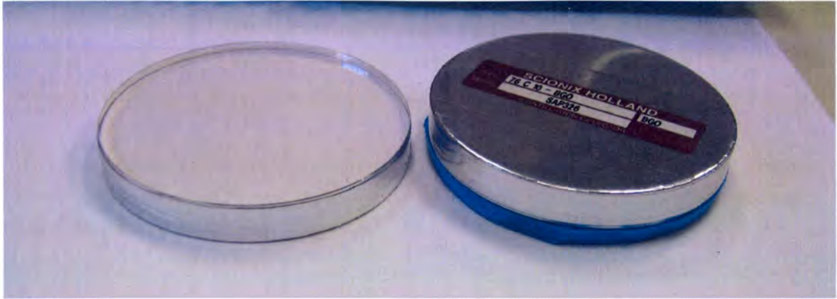
Figure 3.6: BGO Scintillation Crystal
