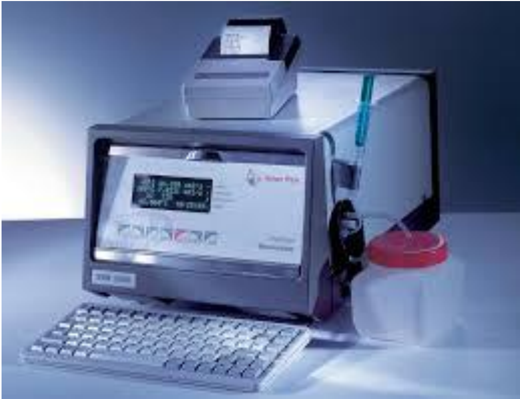
Figure 3.3: Anton Paar Stabinger Viscometer SVM3000.
