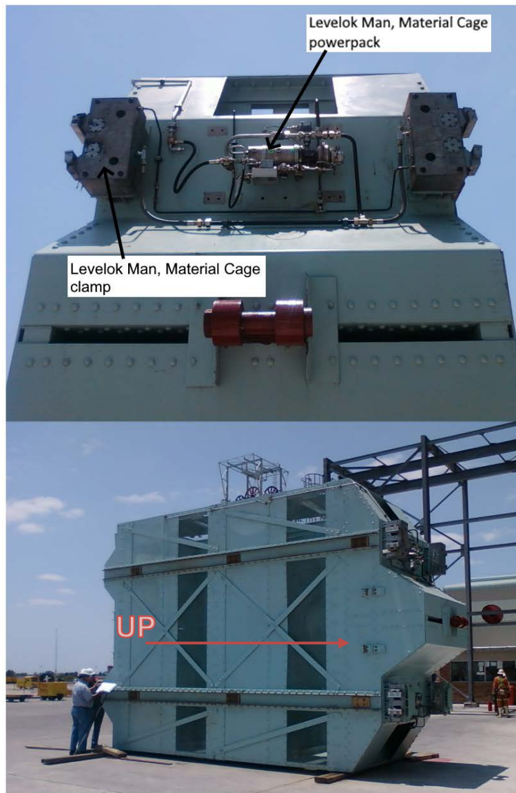
Figure 3: Illustration of the roof of a man, material cage, to demonstrate where the Levelok man, material cage system components are mounted [4] [5] (Note: The conveyance in the illustration is placed on its side. During the installation of the conveyance in the shaft, a “tip-and-tail” maneuver is used to orientate the conveyance vertically.).
