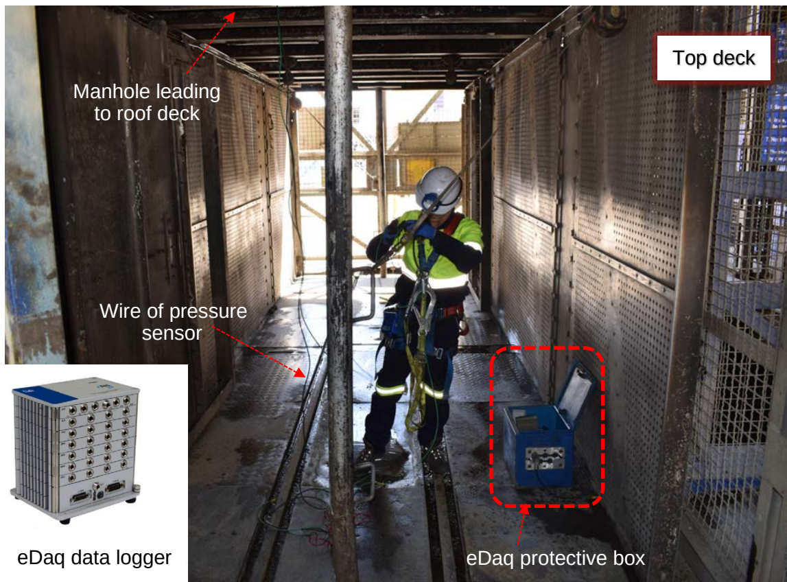
Figure 113: Illustration of the top deck where the eDaq [53] equipment was placed for data logging during the “slide” tests [47].
