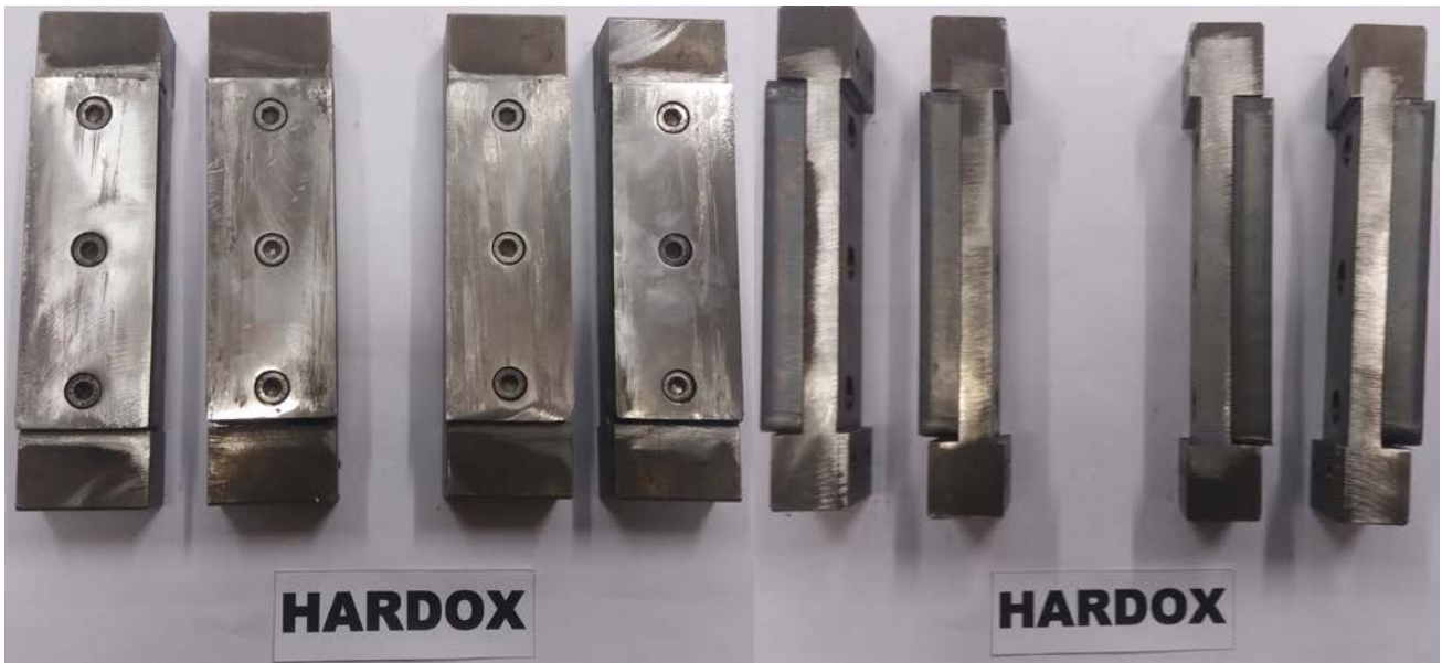
Figure 143: Friction test model set 2, Industrial lining friction shoe inserts with Hardox 900 friction insert [58].
