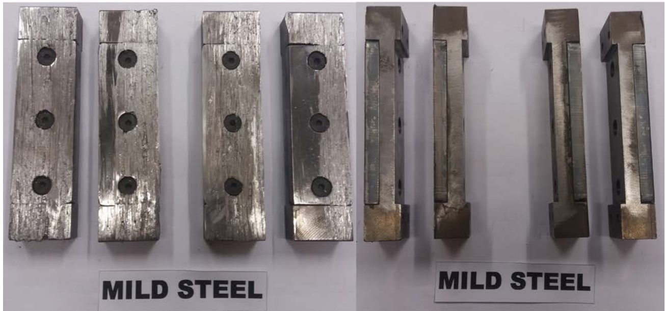
Figure 145: Friction test model set 3, Industrial lining friction shoe inserts with mild steel 355J friction insert [58].
