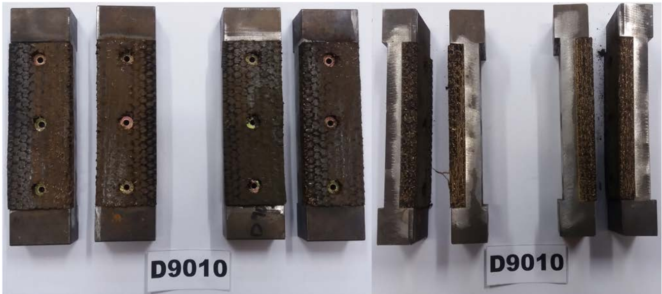
Figure 149: Friction test model set 5, Industrial lining friction shoe inserts with D9010 friction inserts [58].
