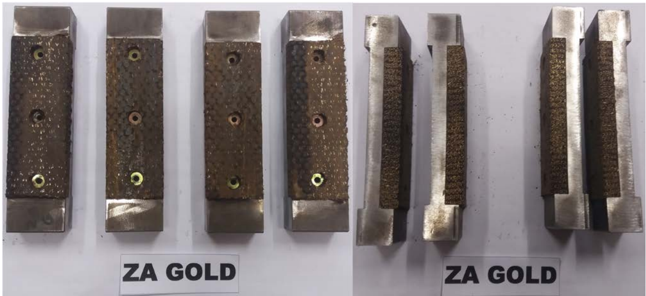
Figure 147: Friction test model set 4, Industrial lining friction shoe inserts with ZA Gold friction insert [58].
