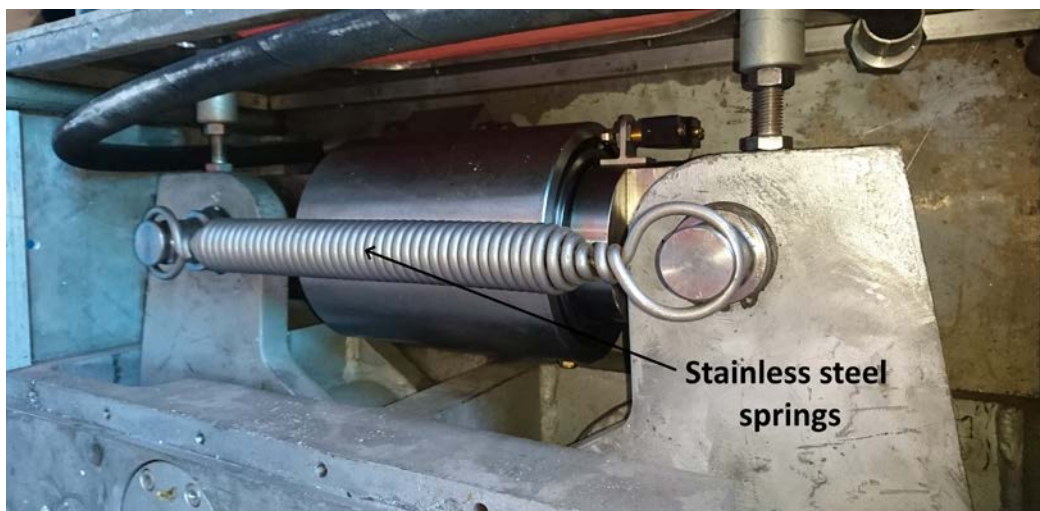
Figure 27: Illustration of the stainless steel springs that are provided in each clamp to assist with the retracting of the hydraulic clamps [47].
