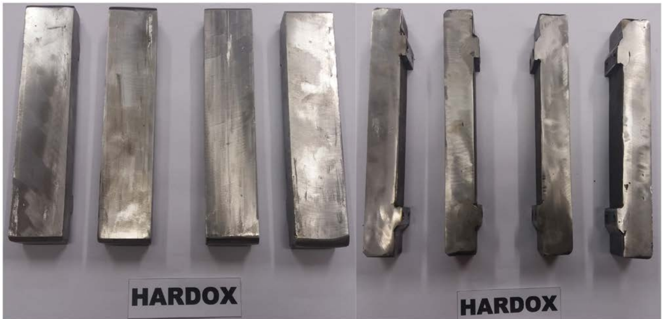
Figure 141: Friction test model set 1, Flat-faced friction shoe inserts made of Hardox 900 steel [58].
