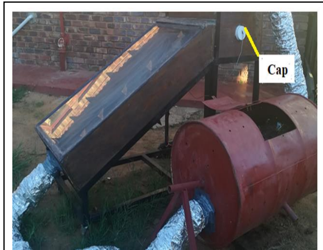
Fig 3. 8: Air inlet sealed with cap.
