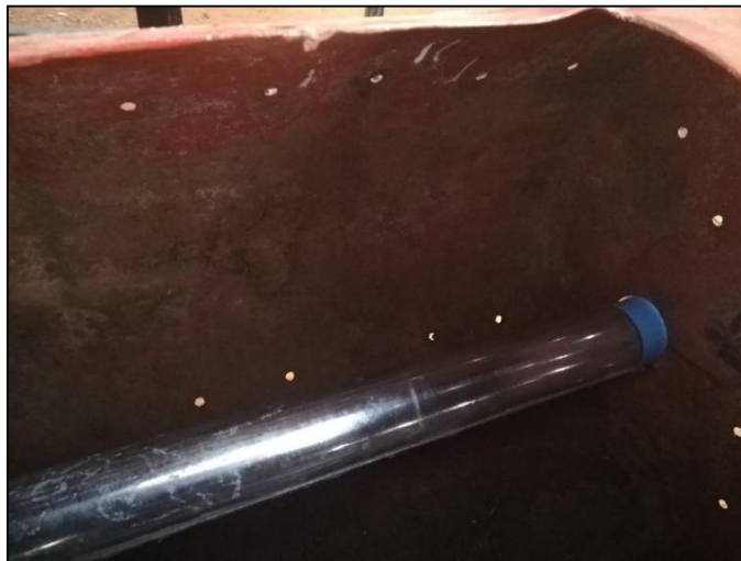
Fig 3. 9: Galvanized iron pipe at the centre of the bioreactor.
