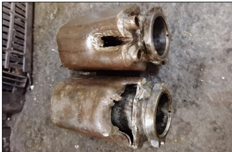
Figure 14: Example of intentional wastage: Broken (tampered) rock-drill muffler 9
