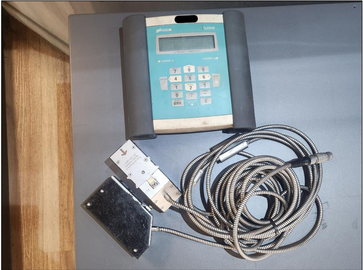
Figure 28: Ultrasonic flow meter with transducers
