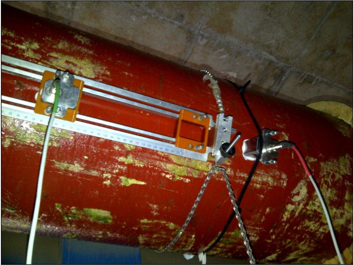
Figure 29: Mine A - ultrasonic flow meter probe mounting
