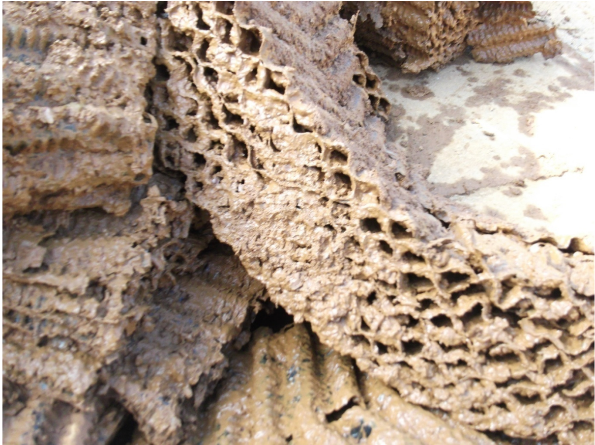
Figure 37: Mine B - existing pre-cooling tower fill material
