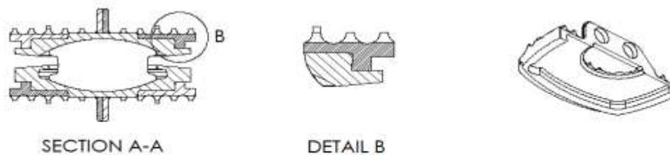
Figure 53: Titanium-PEEK interface, acute angle encapsulating wear body
