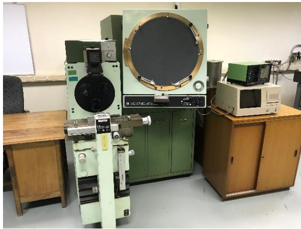
Figure 3-14 – Photograph of the Microtecnica Titanus 6 at Necsca used for the measurement of the longitudinal dimensions and diameters of the fuel rod endcaps
