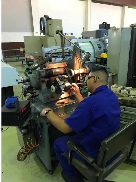
Figure 3-13 – Image of a Necsa artisan using the EWAG precision grinder to cut the endcaps to size.
