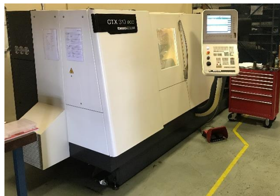
Figure 2-10 – DMG Ecoline CTX 310 eco Turret Lathe
