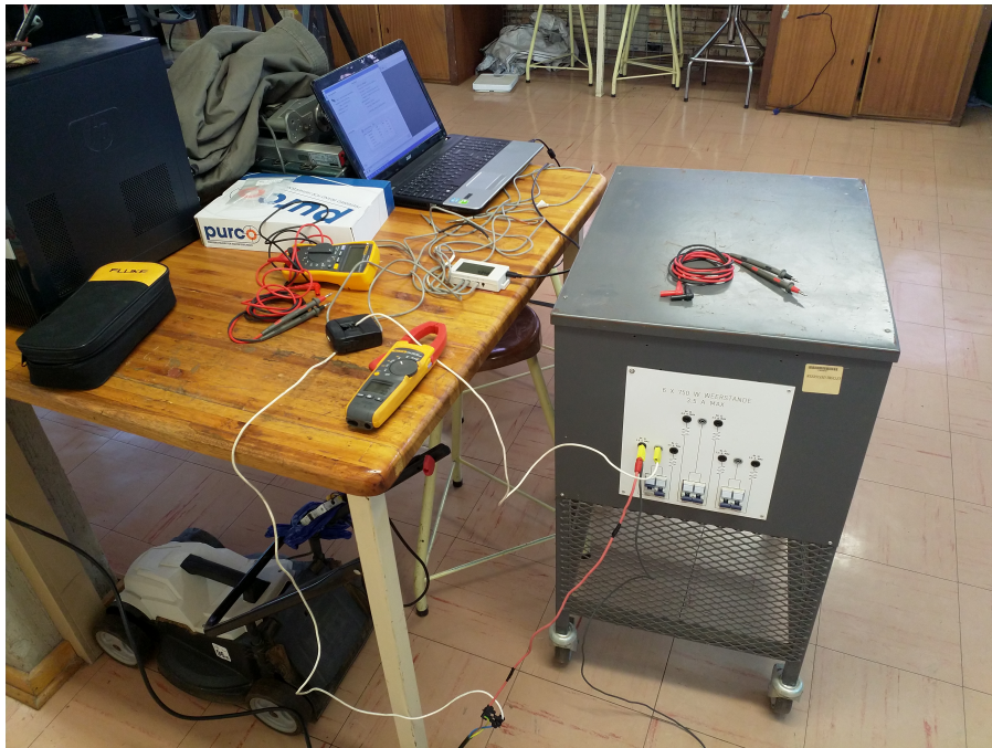
FIGURE A.3: Electrical ammeter calibration against reference meters.
