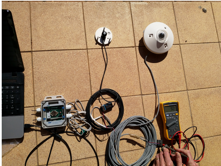
FIGURE A.1: Pyranometer verification against reference pyranometer.
