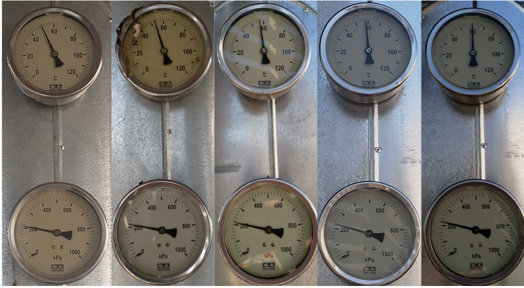
FIGURE 3.10: Temperature stratification between warmest and coldest tank during a 'charge' cycle.
