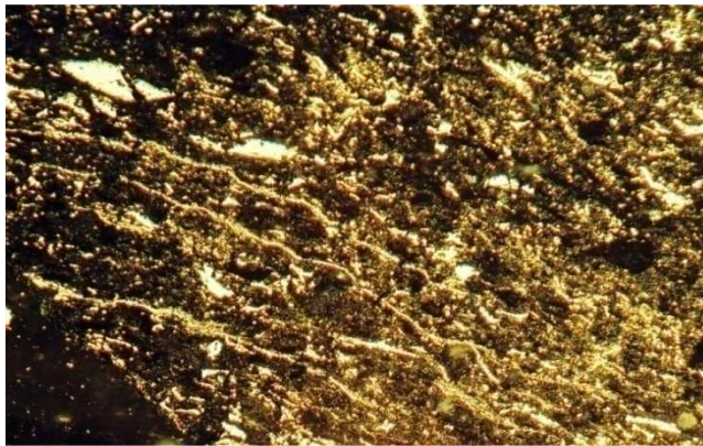
(v) Fine inertinite particles associated with clay minerals from carbominerite in the parent coal
