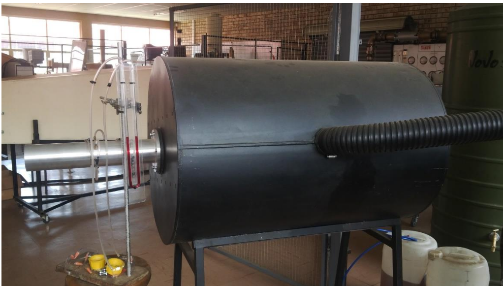
Figure 39 - Air drum used to minimise pulses in air flow measurements
