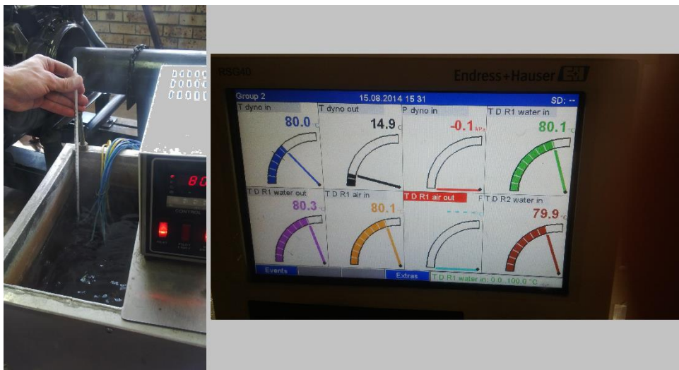
Figure 33 - Thermocouple calibration at 80°C
