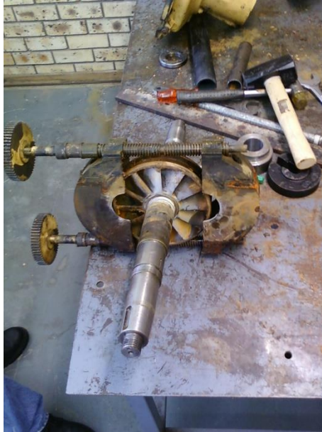
Figure 8 - Water brake dynamometer rotor with sluice gates
