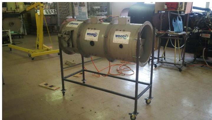
Figure 24 - Cooling fan for radiator
