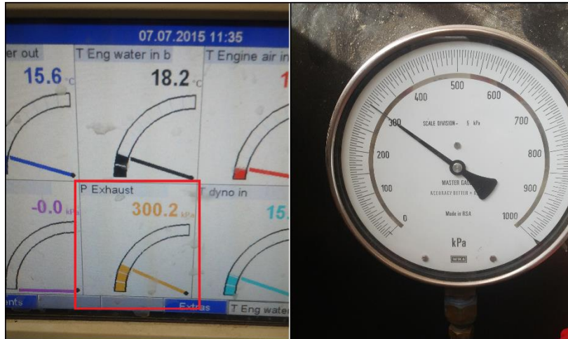
Figure 36 - Pressure transducer calibration at 300 kPa
