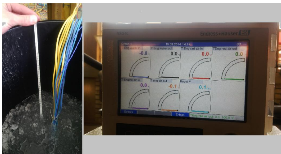
Figure 32 - Thermocouple calibration at 0°C
