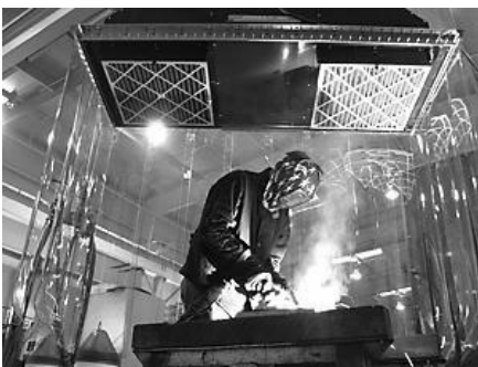
Figure 6: Fume extraction through an overhead canopy hood.
