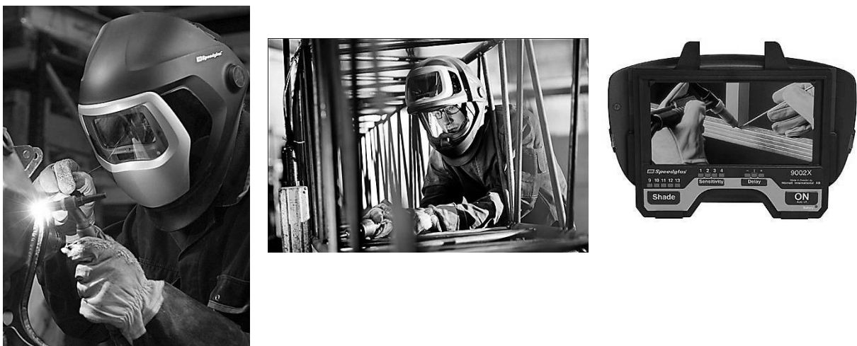
Figure 9: Speedglas™ welding shield worn during welding (left), non-welding tasks (middle) and the vision of the welding shield from the inside (right). Cost of Speedglas™ welding shield: From R1986.60.
