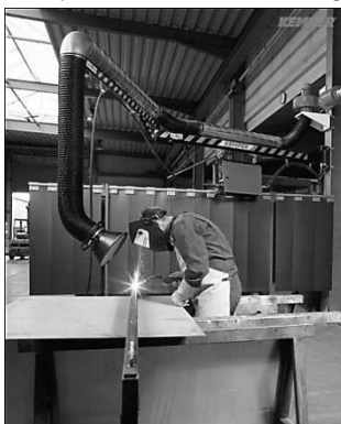
Figure 2: Extraction arm and crane extracting fumes away from the welder.
