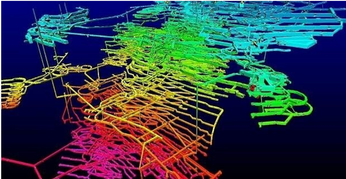
Figure 2-8: Ventsim simulation package – 3D network example [59]
