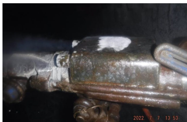
Figure 1-5: Ice formation on compressed-air drill. 6
