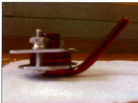
Photo C.1: Amber Franz diffusion cell, with the donor and receptor compartments clamped together with a metal clamp.
