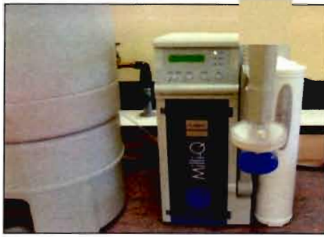
Photo C.4: Milli-Q water purifying system.
