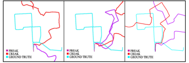
Fig. 7. Odometry with ORB detecting 500, 1000 and 2000 Key-points
