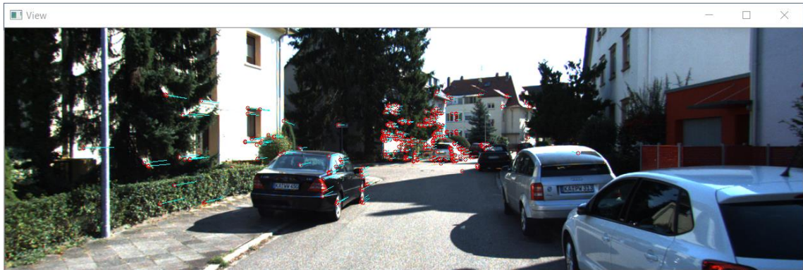
Figure 4.8 - Monocular Visual Odometry Feature Matching in the KITTI [5] dataset 00 where Red circles represent newly observed landmarks, and Cyan lines are drawn towards the landmark's previous position
