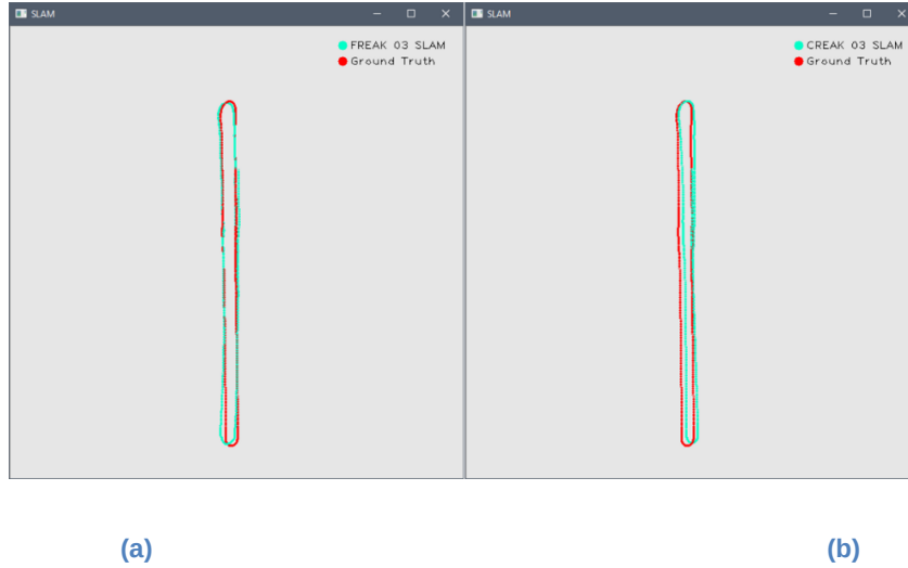
Figure 4.19 - (a) FREAK EKF-SLAM and (b) CREAK EKF-SLAM Trajectory for Dataset 03
