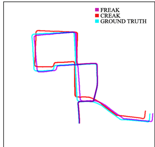
Fig. 8. Odometry with FAST detecting roughly 5000 Key-points
