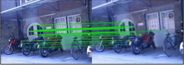
Fig. 13. Bikes 1/6 Blur FREAK results (167 Matches, 166 Correct)
