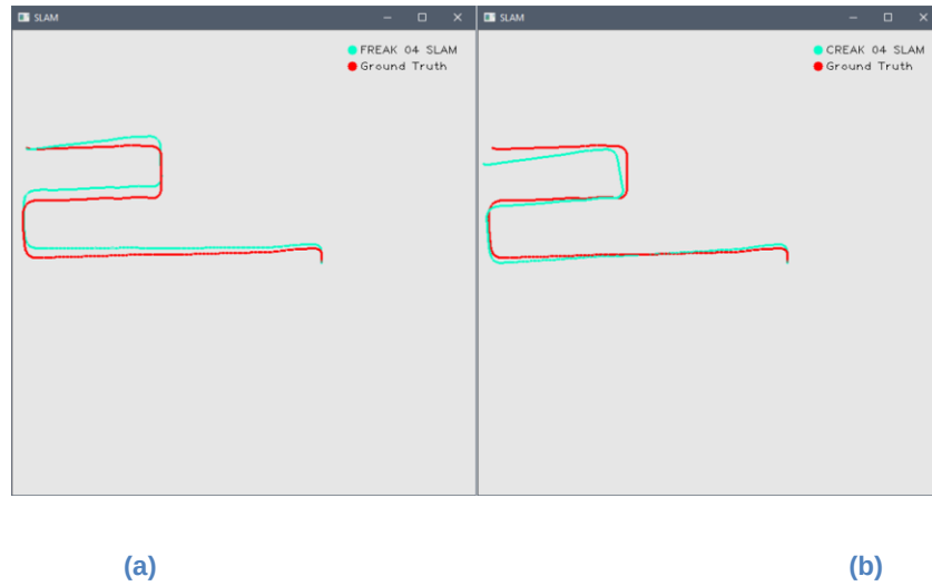
Figure 4.20 - (a) FREAK EKF-SLAM and (b) CREAK EKF-SLAM Trajectory for Dataset 04
