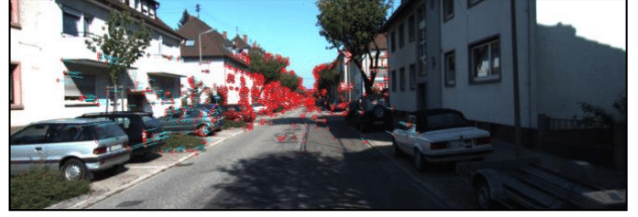
Fig. 6. Detected and Tracked Key-points using the CREAK descriptor
