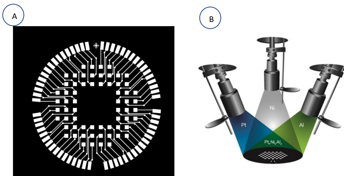
Figure 1. Circuit layout on Si-SiO 2 wafer (a) and the combinatorial PVD system used for vacuum sputtering of thin film electrocatalysts (b)
