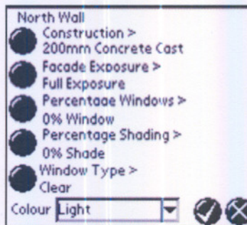
Figure 2-7: North wall interface
