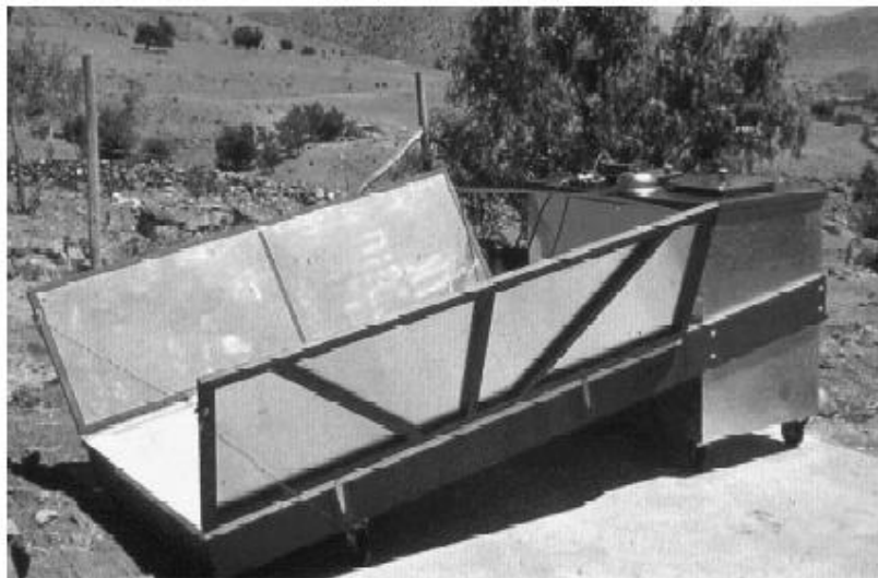
Figure 9: Indirect flat plate collector solar cooker with TES designed by Schwarzer and daSilva (2003)
