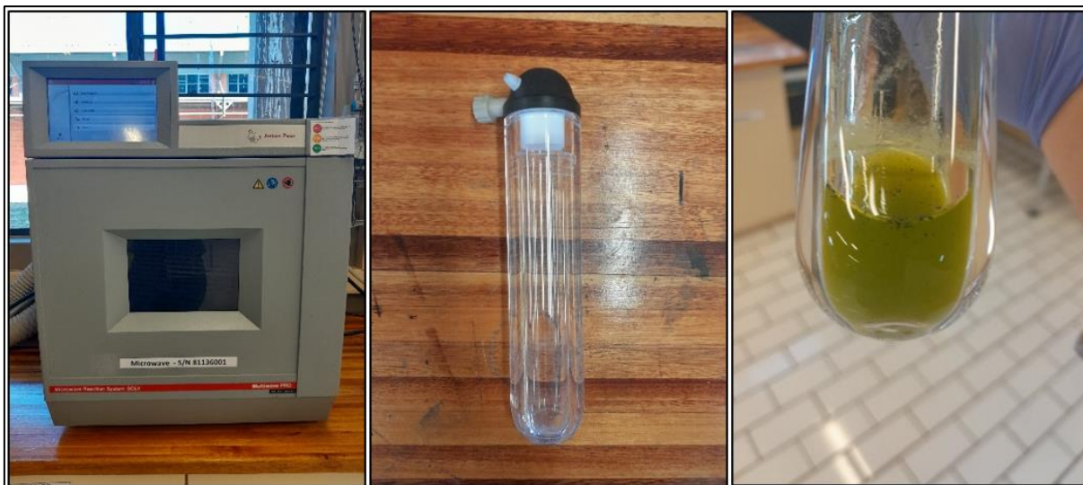
Figure 3-4: Microwave digester (left), lip-sealed digestion vessel (middle), and digested sample (right)
