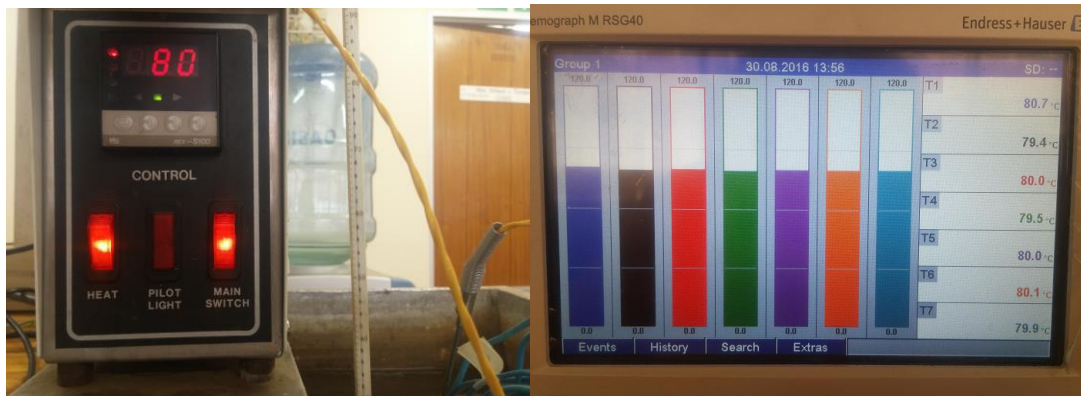
Figure 117: Calibration of type K thermocouples inside a control heat bath
