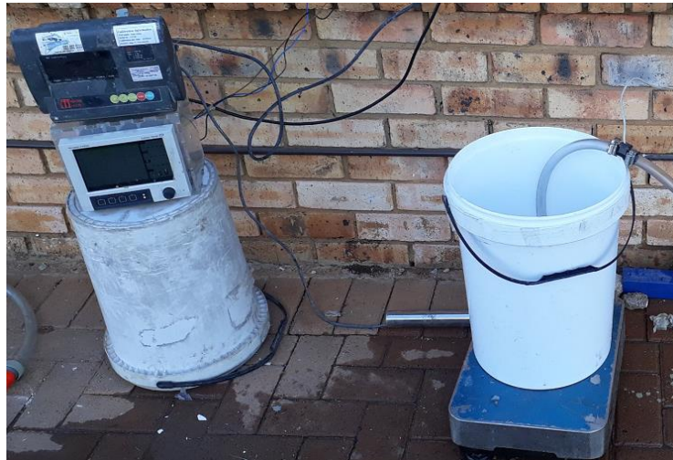
Figure 114: Water flow sensor calibration
