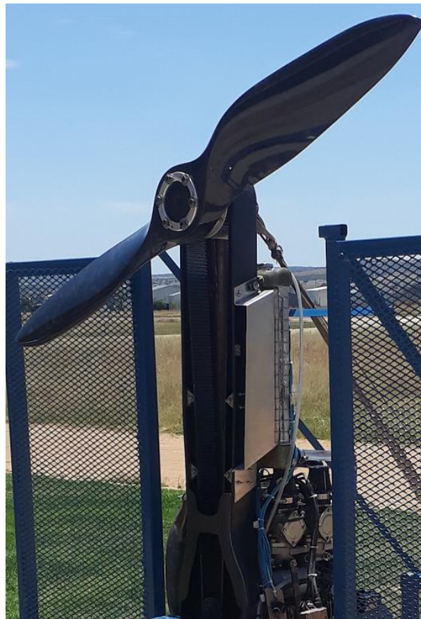
Figure 100: Radiator scoop installed on the pylon
