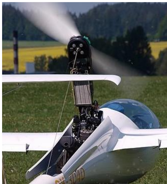
Figure 1: Example of a retractable self-launching sailplane (HPH, 2018)
