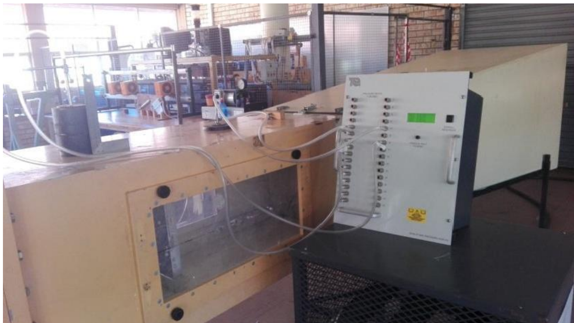
Figure 42: Pitot tube connected to the digital 32-way pressure display unit
