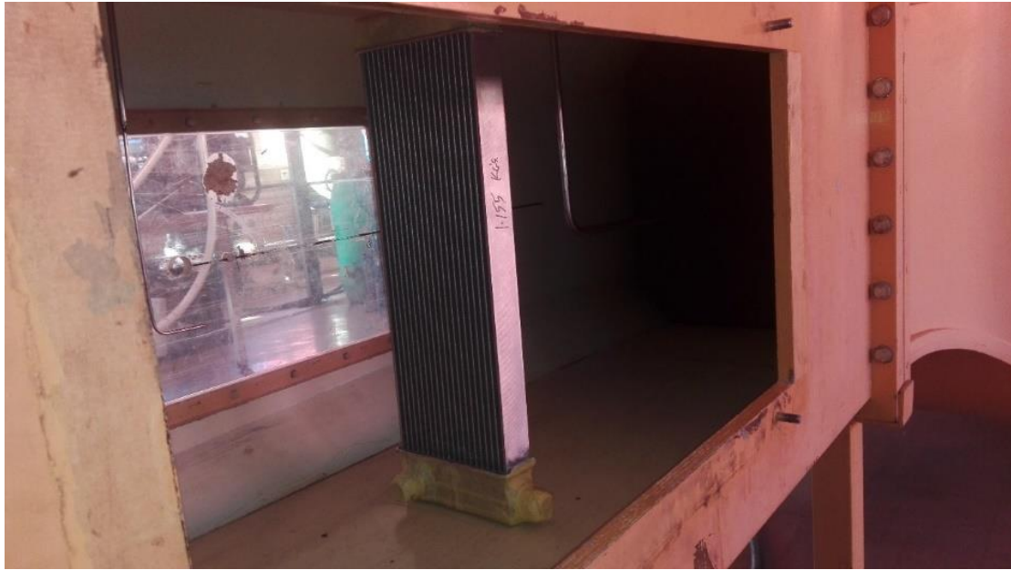
Figure 43: Radiator placement inside the wind tunnel
