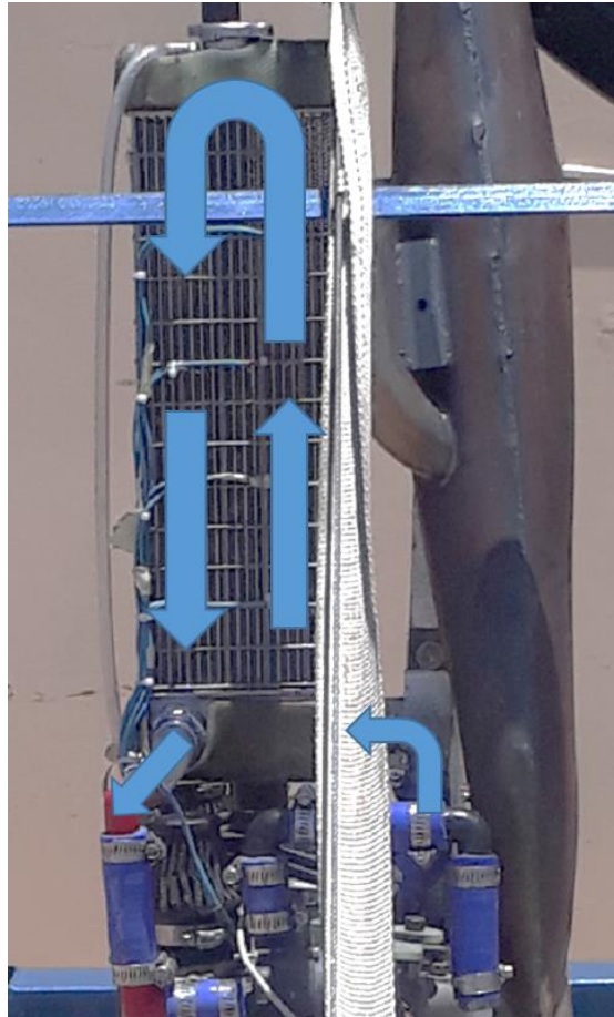
Figure 47: Coolant flow path through the double-pass radiator. Flow enters from the right-hand side in the image and exits on the left.
