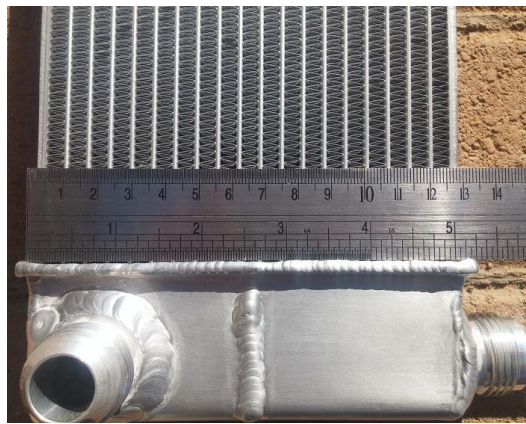
Figure 8: Double pass radiator used in the self-launch system.
