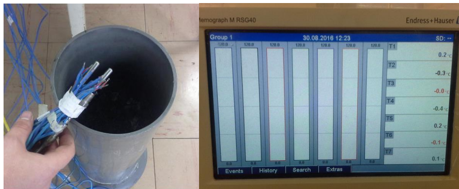
Figure 116: Calibration of type-K thermocouples in ice bath
