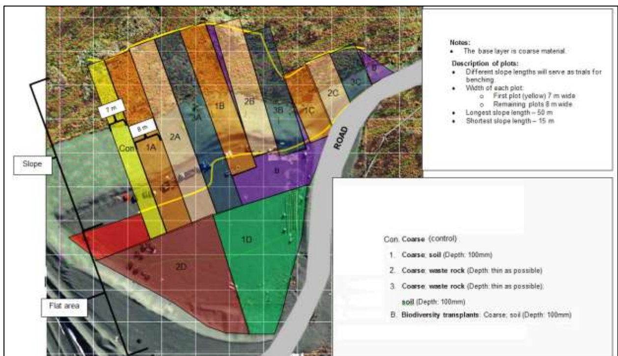
Figure 3-4: Layout and various treatments on rehabilitation trial site 2 (De Beers TSF coarse tailings wall) (adapted from E-Tek Consulting, 2014).
