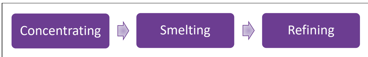
Figure 2: Typical PGM processing flowchart [2]
