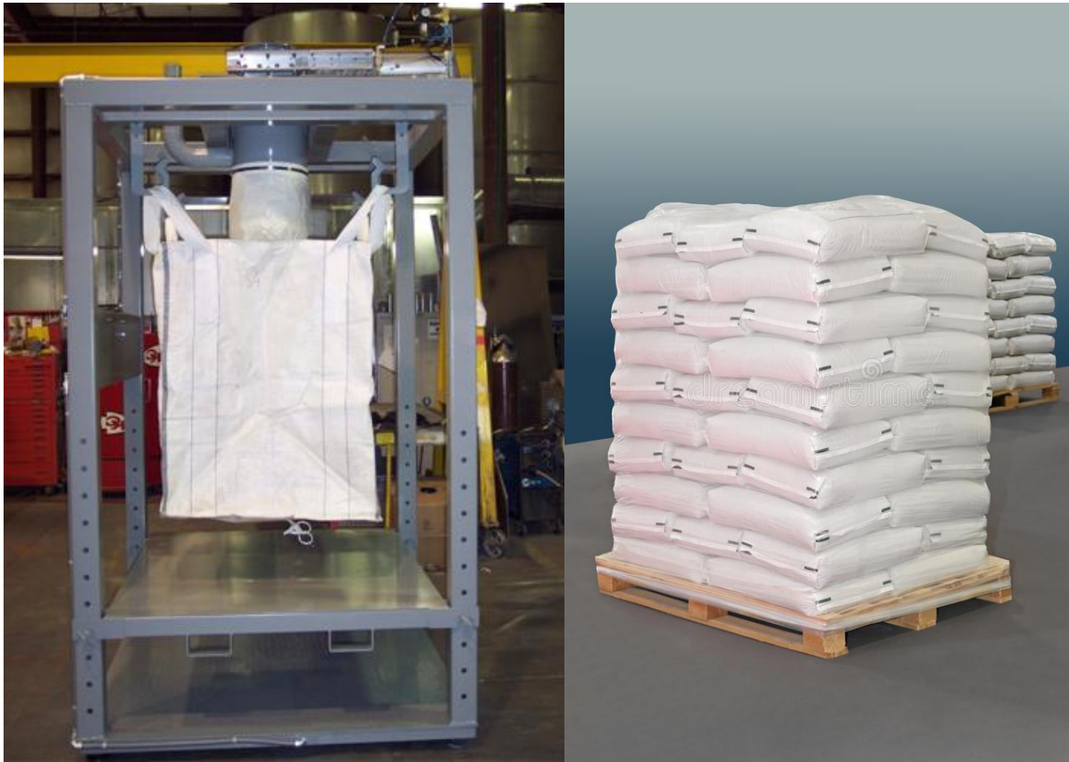
Figure 1-8 Example of Flexible Industrial Bulk Containers (FIBC) bag and a pallet of 20kg bags
