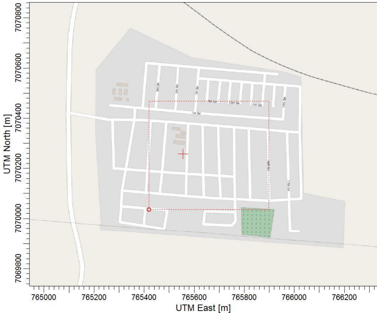
Figure 3-20. Windblown dust as one area source with a total area of 344314.6531m 2
