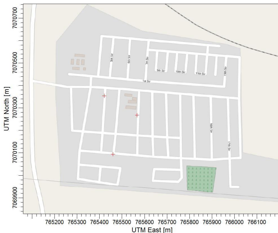
Figure 3-12. Open street map of Kwadela and the three discrete receptors used in all model runs placed at the three monitoring sites
