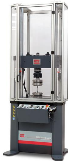
Figure 3-13: MTS 100kN servo hydraulic test bench
