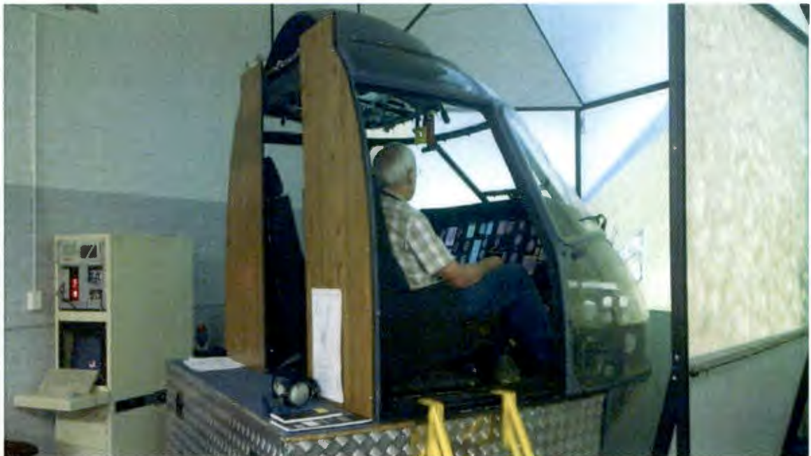
Figure 11: Helicopter hardware-and-pilot-in-the-loop simulation system
