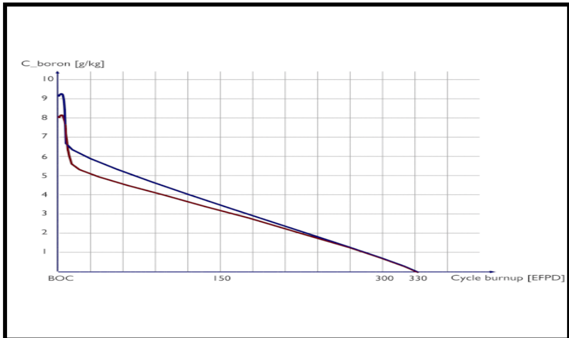
Figure 2-3: The CBC in a core without burnable absorbers (blue curve) and core with burnable absorbers (red curve) (Nuclear-Power, 2017).
