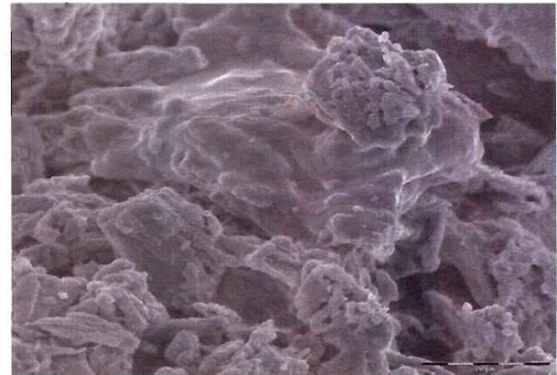
Figure 3.12: Magnified view of a 1% (w/w) Kollidon® SR chitosan granule loaded with ketoprofen.
