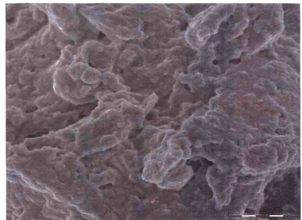
Figure 3.20: Magnified view a 5% (w/w) Kollidon® SR chitosan granule (Kollidon® SR was dissolved in 2-Pyrrolidinone® and ketoprofen dissolved in ethanol prior to granulation).
