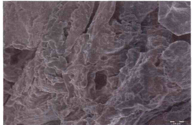
Figure 3.18: Magnified view of a 10% (w/w) Kollidon® SR chitosan granule (Kollidon® SR was dissolved in 2-Pyrrolidinone® prior to granulation).
