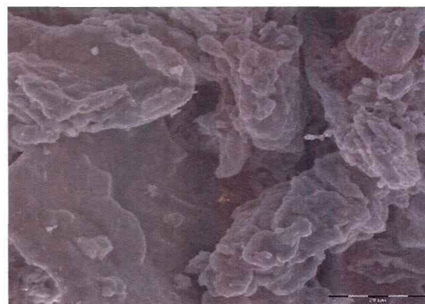
Figure 3.16: Magnified view of a 10% (w/w) Kollidon® SR chitosan granule loaded with ketoprofen.
