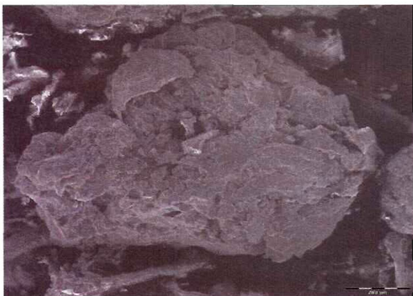
Figure 3.13: Full view of a 5 % (w/w) Kollidon® SR chitosan granule loaded with ketoprofen.
