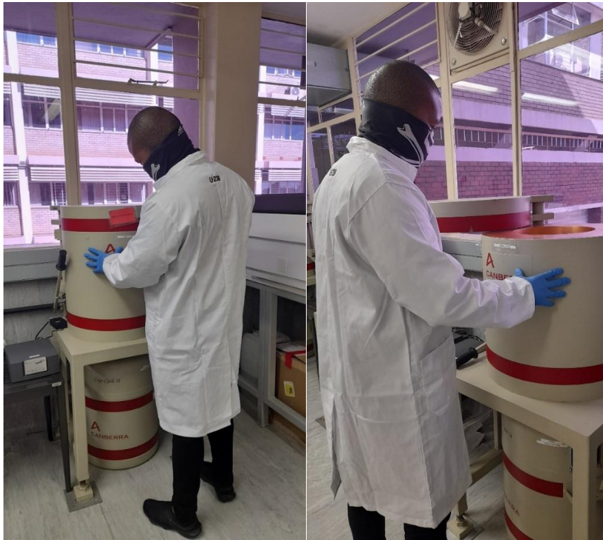
Figure 3. 12: Sediment analysis with Canberra HPGe detector.
