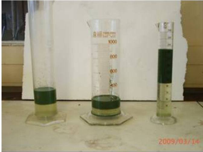
Figure 52: Hartbeespoort Dam microalgae separating to the top of the measuring cylinders after 3.5 hours at a concentration of 3% TSS.
