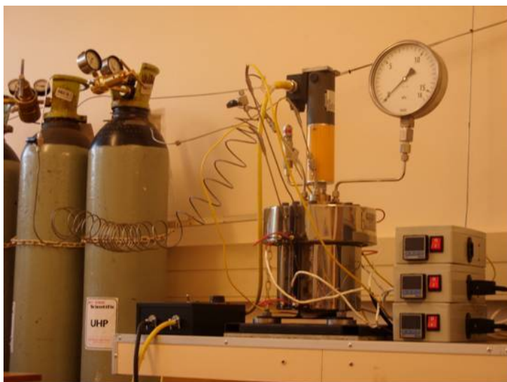
Figure 53: Experimental set-up used by Barnard (2009) to extract oils from Hartbeespoort Dam microalgae, showing the liquefaction autoclave and associated monitoring and regulating equipment.
