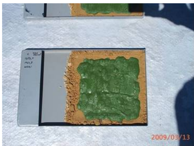
Figure 84: Sun-dried palette of micro-algal biomass from the Hartbeespoort Dam on top of a base of building sand, located on top of the roof of the laboratory at the North-West University at Potchefstroom.
