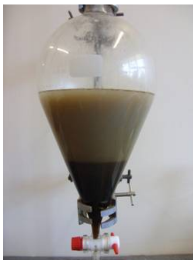
Figure 54: Water-oil-solvent mixture separating into two distinct layers: a top layer of water and micro-algal biomass rests, and a bottom layer consisting of oil and chloroform solvent.
