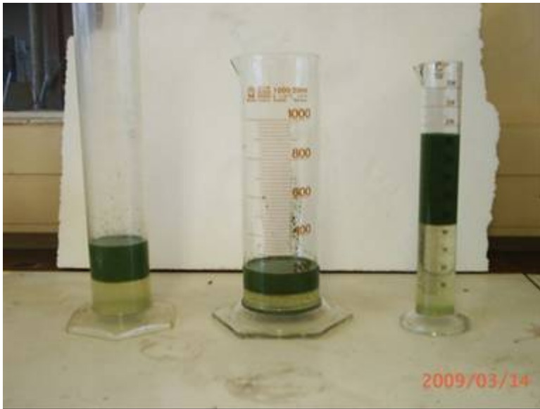
Figure 21: Hartbeespoort Dam micro-algal biomass concentrating at the top of measure cylinders after 24 hours.
