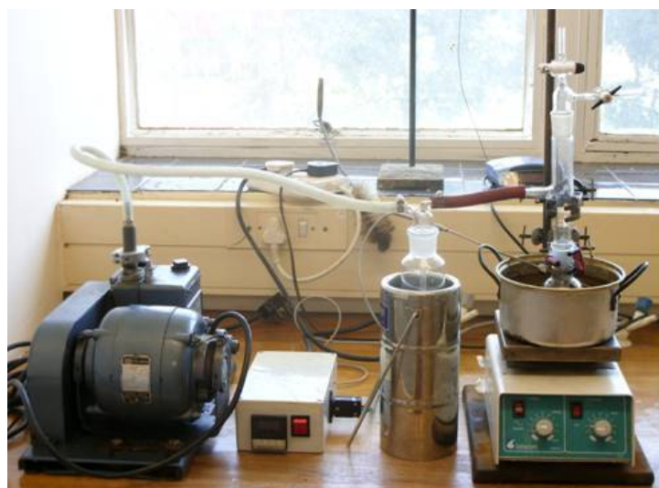
Figure 56: Vacuum distillation set-up used by Barnard (2009) to separate micro-algal oils from the chloroform solvent.
