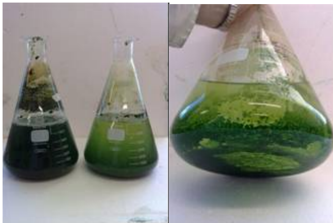
Figure 57: Comparison of two 5-litre Erlenmeyer flasks with cultivated microalgae from the Hartbeespoort Dam, showing a well-mixed flask on the left, and the concentrated microalgae that settled to the bottom of the right flask after 24 hours.
