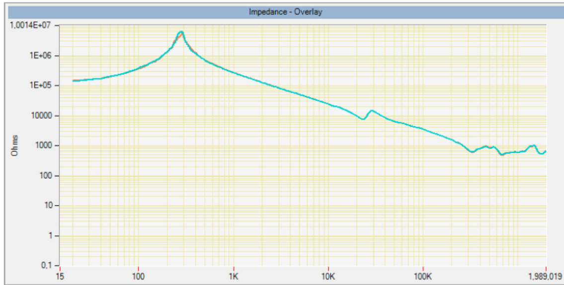
Fig. 3-55: The impedance amplitude of the SFRA done on the transformer in question with the LV winding open
