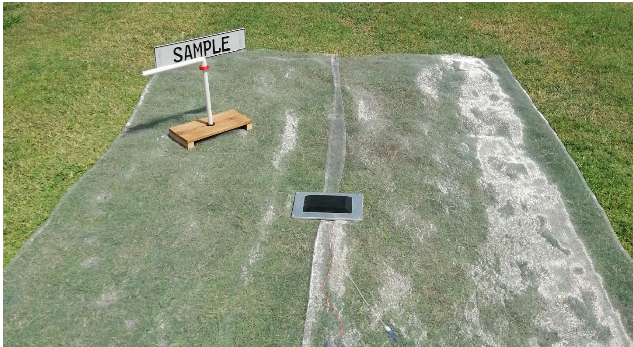
Figure 50: In-road antenna test setup
