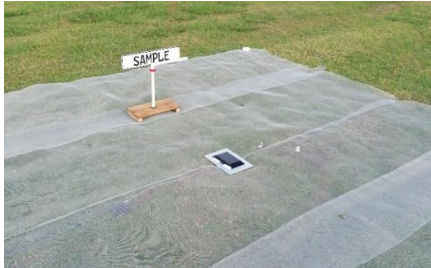
Figure 58: Required RFID antenna ground plane
