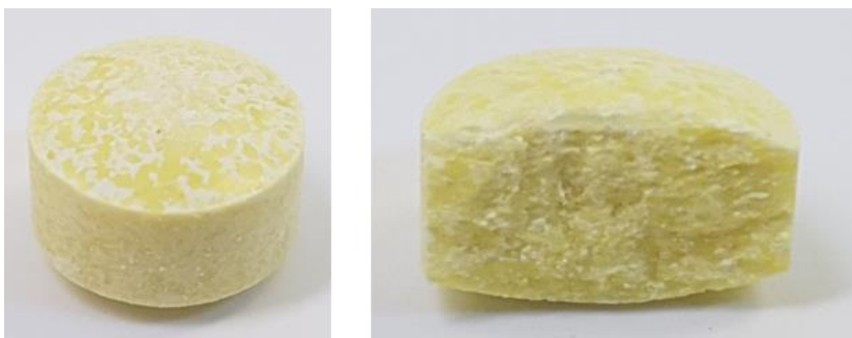
Figure E.3: SA0.75M1 external (left) and internal (right) surface morphology image
