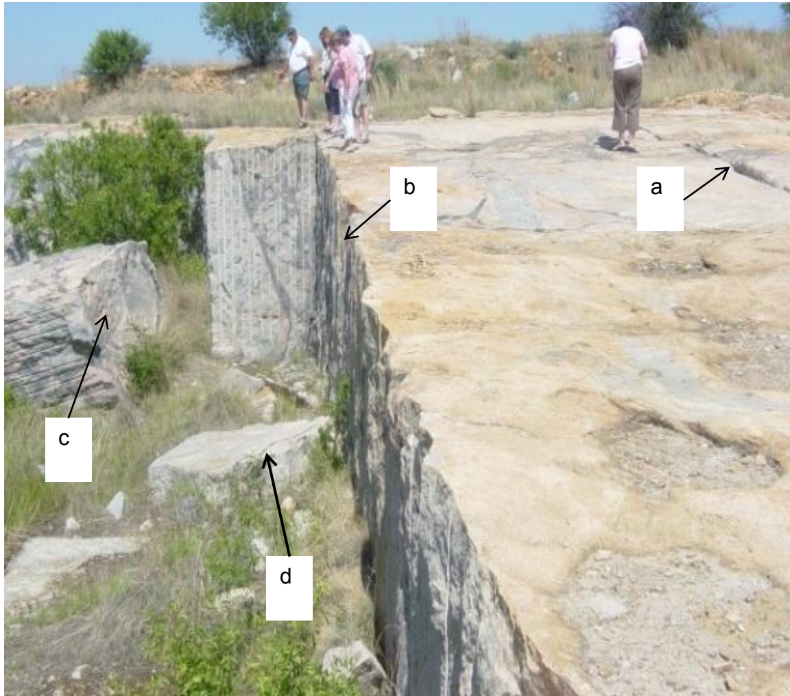
Figure 45. In this photograph a full mining sequence from (a) thermal lance cutting, to (b) percussion drilling, and (c) blasting is displayed at the Salvamento Quarry. To the left of the quarry face block (d) just tipped over, while block (c) was lifted out of its original position by explosives.
