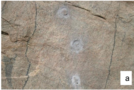
Figures 47a and b. Scientific researchers start to heed the concepts of conservation when the cores of diamond drilling were returned and cemented back in the quarry wall at Salvamento.
