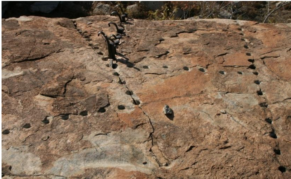
Figure 53. The commonly used square grid implemented to quarry the granite blocks was modified (as can be seen from the percussion holes in the picture) to cut out unwanted structural features and/or to make use of an existing joint system to obtain solid blocks.
