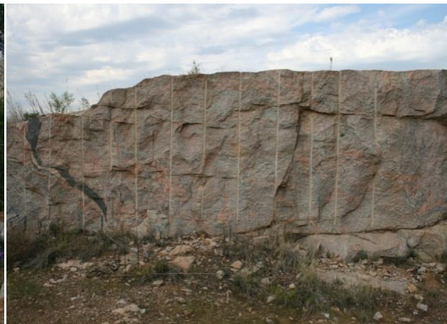
Figure 40. Markings left by percussion drilling holes, which are loaded with dynamite to crack the granite (GQ8, Kopjeskraal 517).
