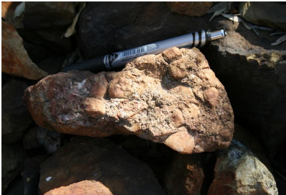
Figure 26. The Yellow Reef/Rous Series or Red Reef/Main Reef observed on the stockpile on Rooderand 510IQ. This reef is a small to medium size pebble matrix supported conglomerate.
