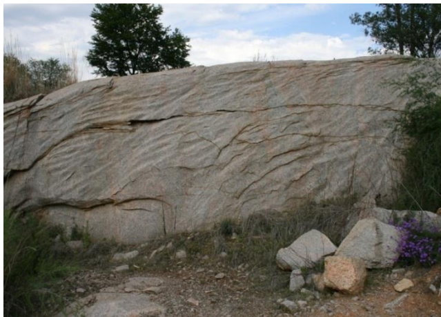
Figure 39 Thermal lance grooves clearly visible on a quarry face (GQ8, Kopjeskraal 517).
