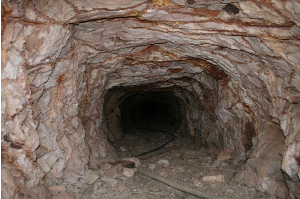
Figure 72. Looking down the decline, RO1, on Rooderand 510IQ. Of general concern is the presence of the plastic water pipes indicating extraction of water in the not too distant past.
