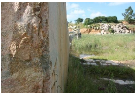
Figure 41. The flat surfaces of two dimension stone blocks from the quarry, GQ8, on Kopjeskraal 517 that were cut with diamond wire.
