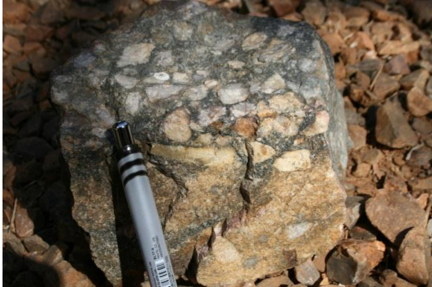
Figure 16. A fresh exposure of the Amazon Reef from Buffelskloof 511IQ. This sample consists of poorly rounded milky quartz pebbles in a dark fine-grained matrix.
