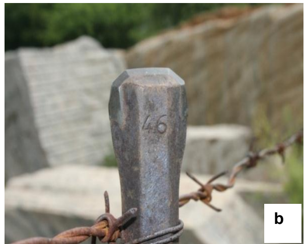
Figure 43. (a) Ignition cord used to ignite dynamite candles, still dangling from drill holes at the GQ8 quarry on Kopjeskraal 157 and (b) jumper rods, used to do percussion drilling, still visible in some drill holes at the same quarry.
