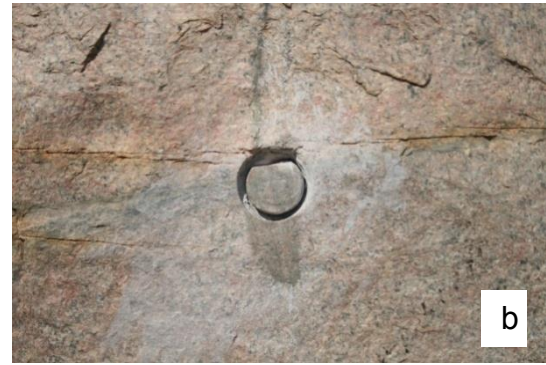
Figures 47a and b. Scientific researchers start to heed the concepts of conservation when the cores of diamond drilling were returned and cemented back in the quarry wall at Salvamento.
