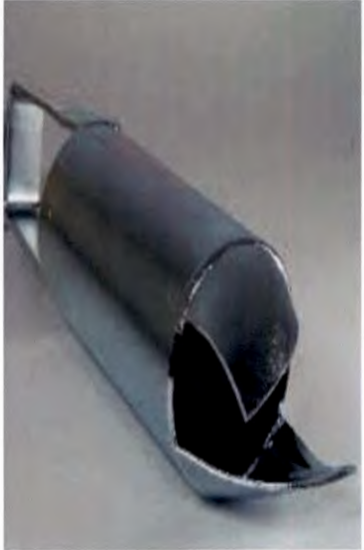
Figure 3.2: A manual auger for extraction of soil samples (AMS samplers)
