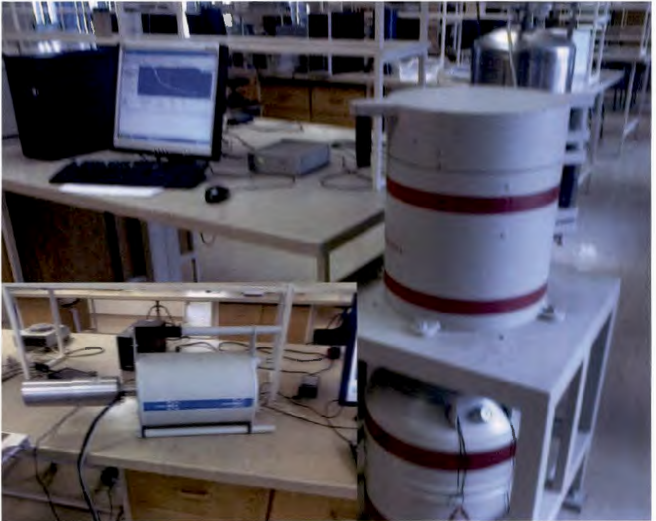
Figure 2.5: Two gamma detectors and the gamma spectroscopy set up
