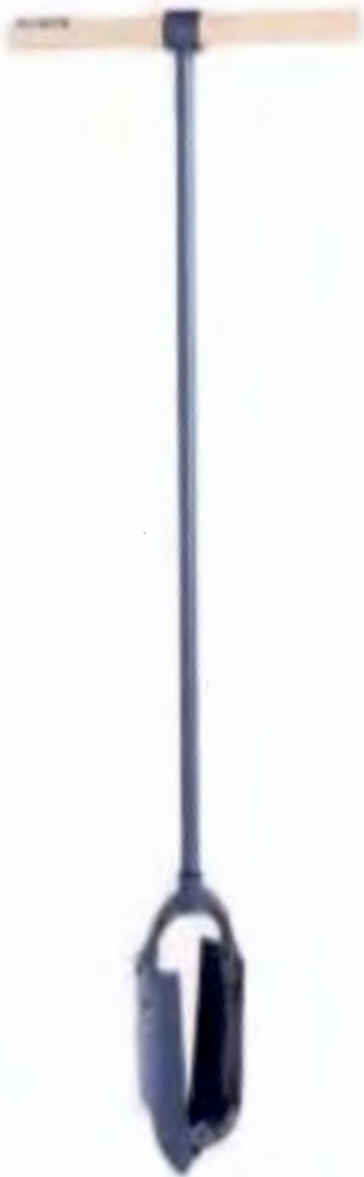
Figure 3.2: A manual auger for extraction of soil samples (AMS samplers)
