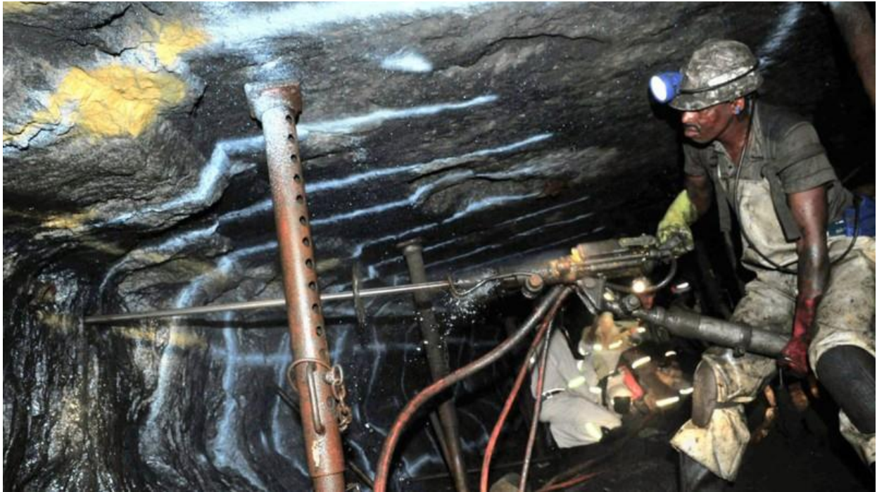
Figure 11: Rockdrill operator drilling a hole with a pneumatically operated rock drill where explosives will be placed 7
