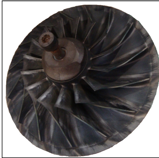
Figure 2 – Photo of an impeller of a centrifugal compressor 1
